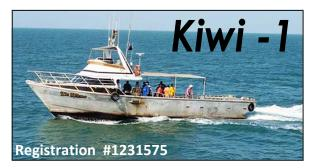
Length:16.47m • Beam:5.2m • Draft:0.8m • Gross Tonnage:25.0 • Net Tonnage:26 • Cruising Range 400 nmi • Cruising Speed:20 knots • Fuel Capacity:3000lt • Main engines:2 x Detroit 8V 92TA DDEC - 1560 hp • Propulsion:2 x Hamilton 362 Jets
