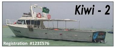
Length:15.2m • Beam:4.2m • Draft:0.6 m • Gross Tonnage 18.0 • Net Tonnage:11.5 • Cruising Range:300 nmi • Cruising Speed:19 knots • Fuel Capacity:2000 It • Main engines:2 x Detroit 6V 92TA - 1100 hp • Propulsion 2 x Hamilton 362 Jets
