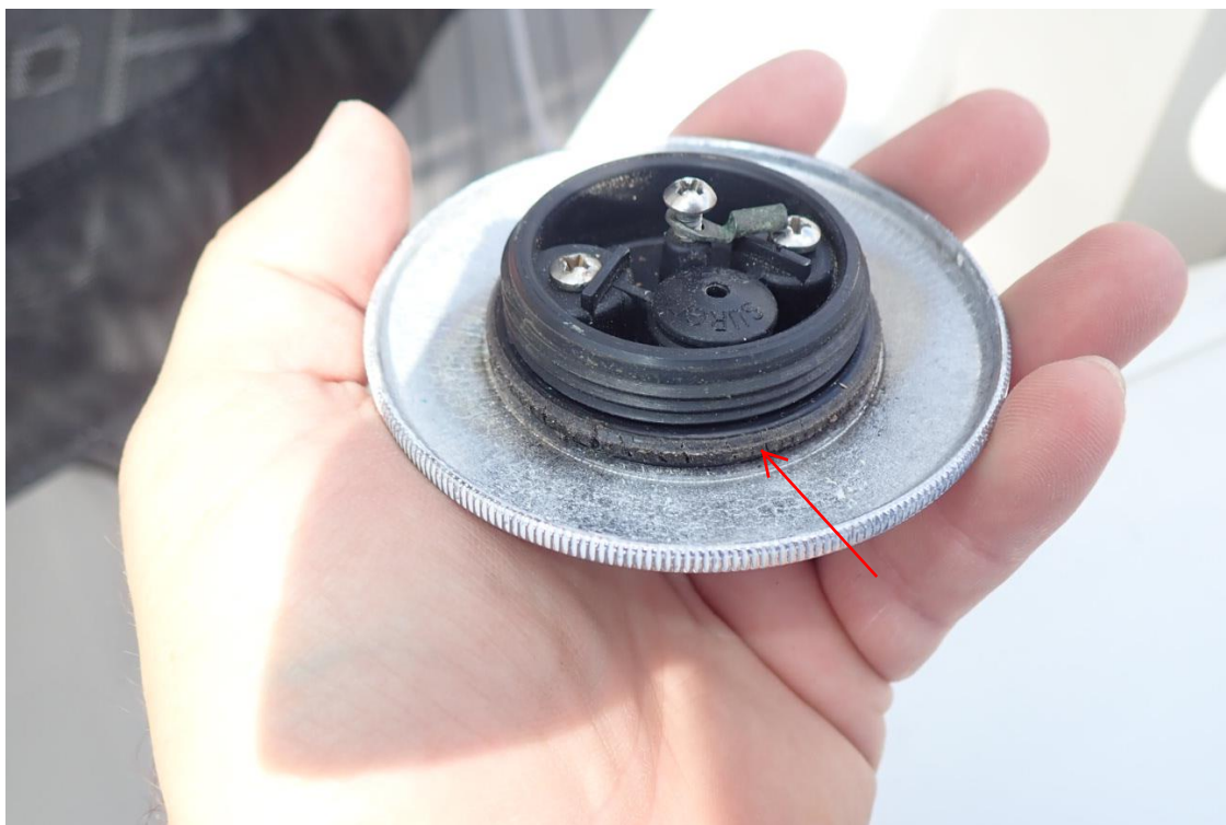
46. Fuel cap O-ring worn
