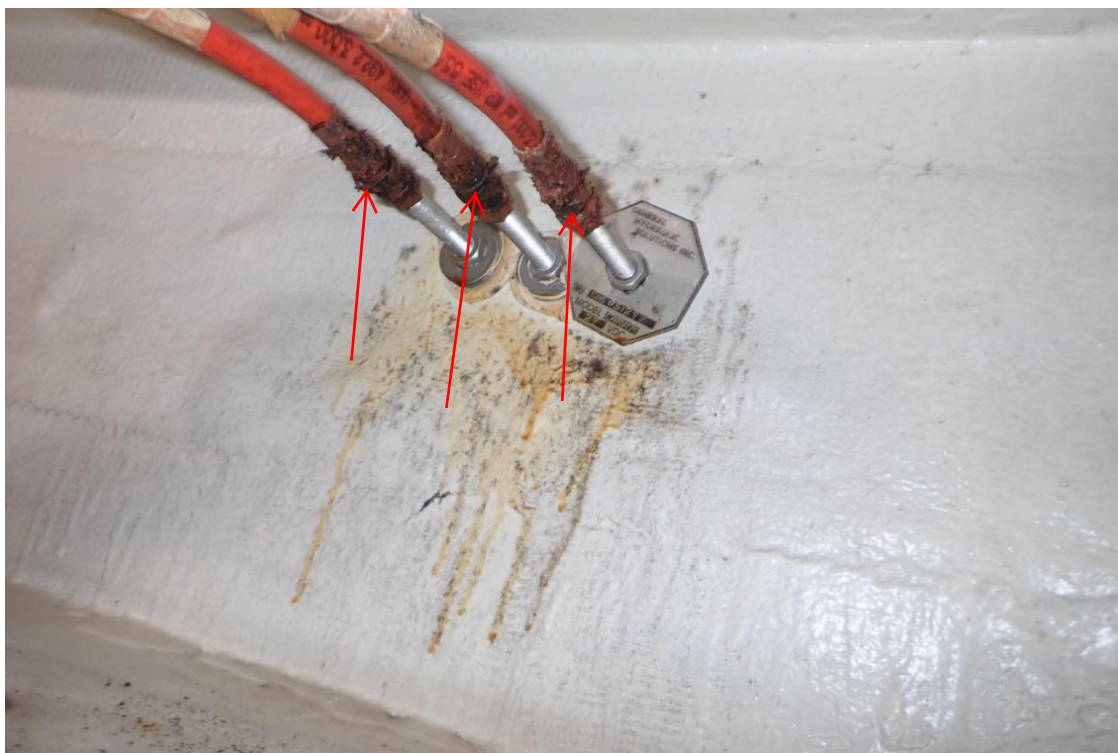
31. Swim platform hydraulic fittings corroding
