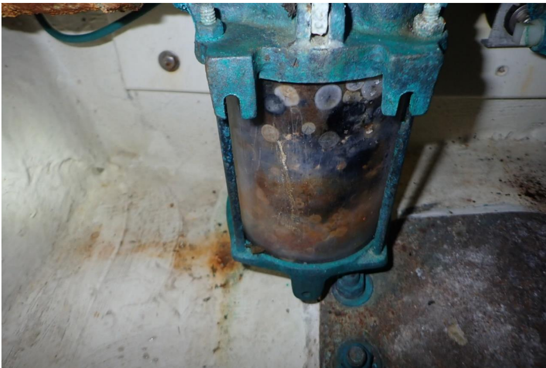
23. Air conditioner sea strainer fouled
