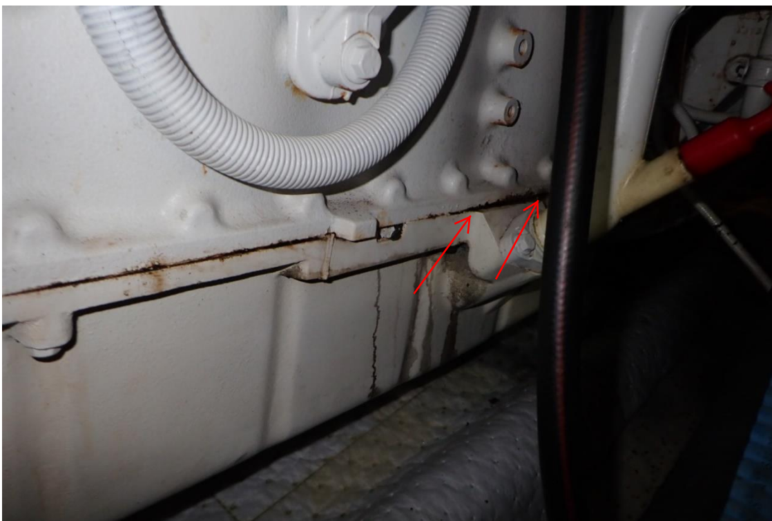
14. Starboard engine oil pan gasket leak
